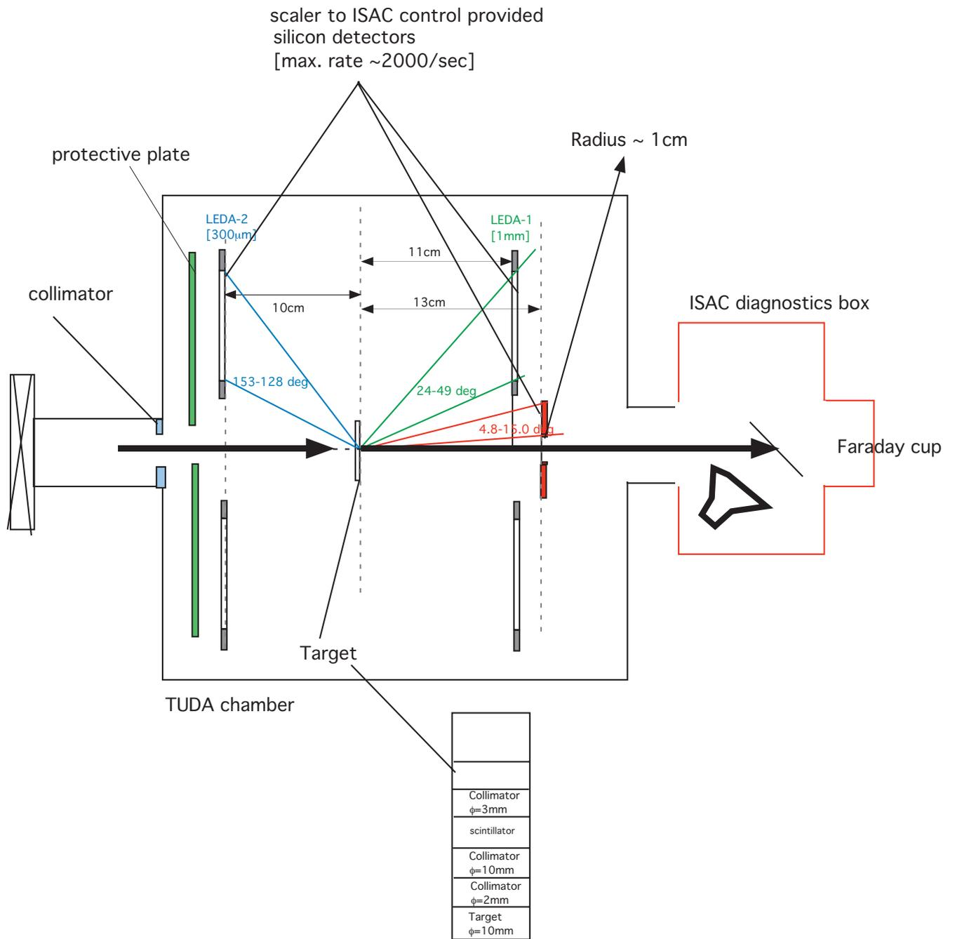
Figure 1: Schematic depiction of the E1057 setup.
