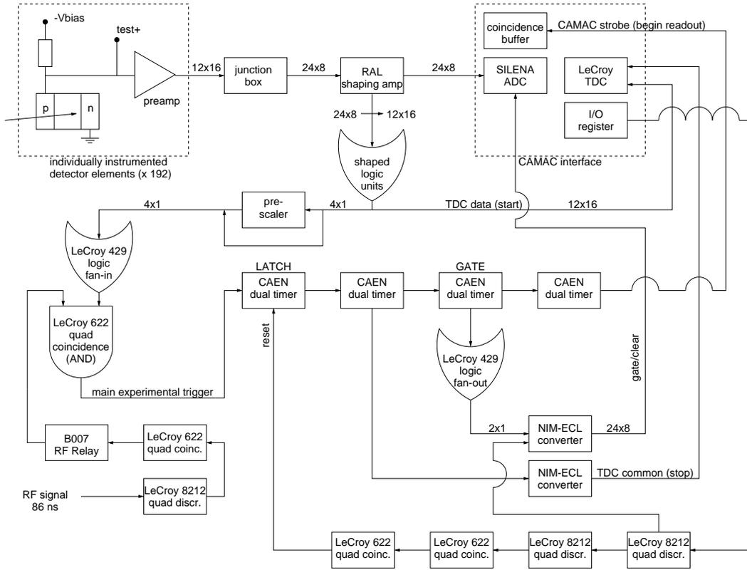
**Figure 5.4:** Schematic of  $^{21}\text{Na}+p$  experiment electronics setup.
