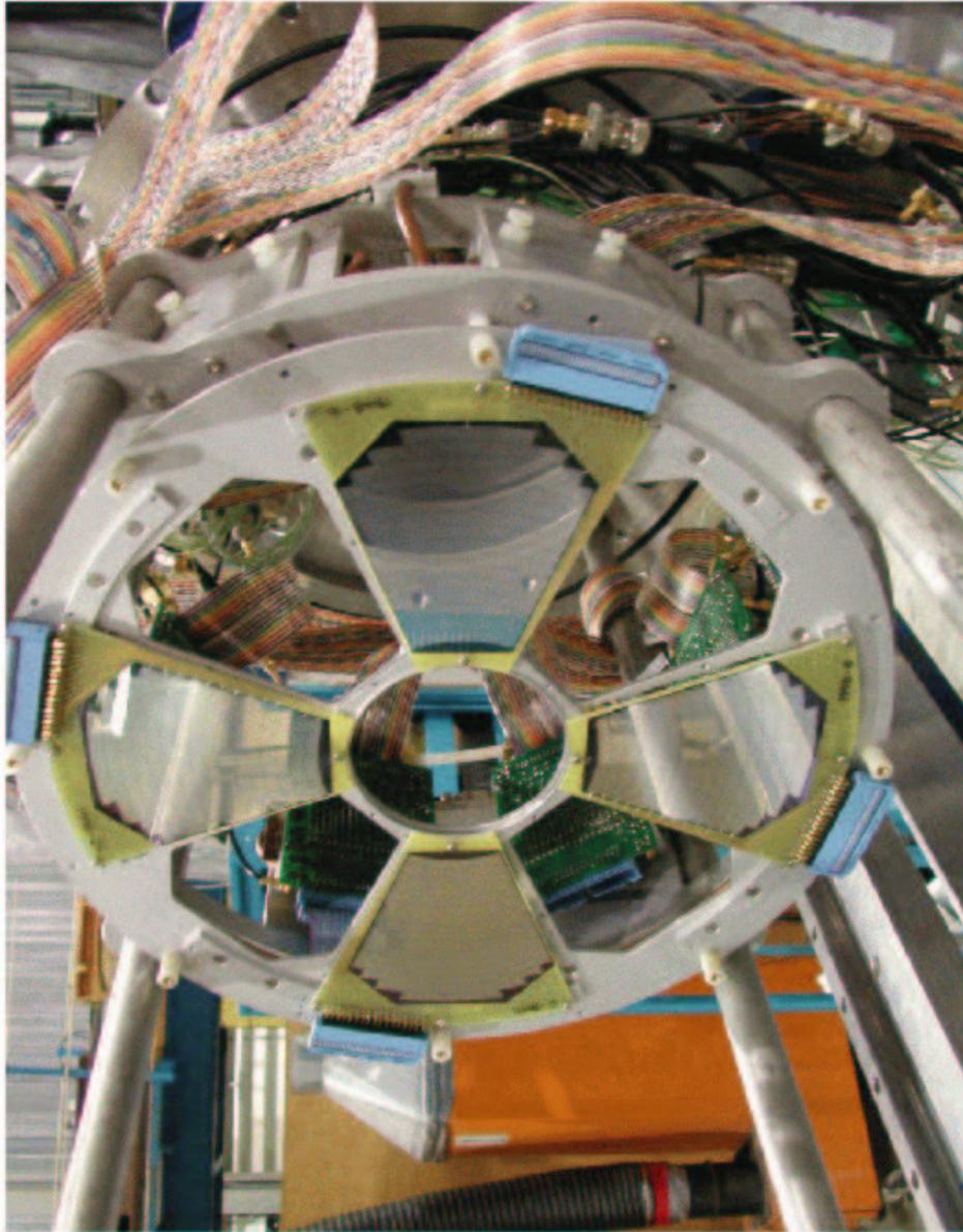
**Figure 5.3:** Photograph of four LEDA detector segments withdrawn from TUDA chamber.
