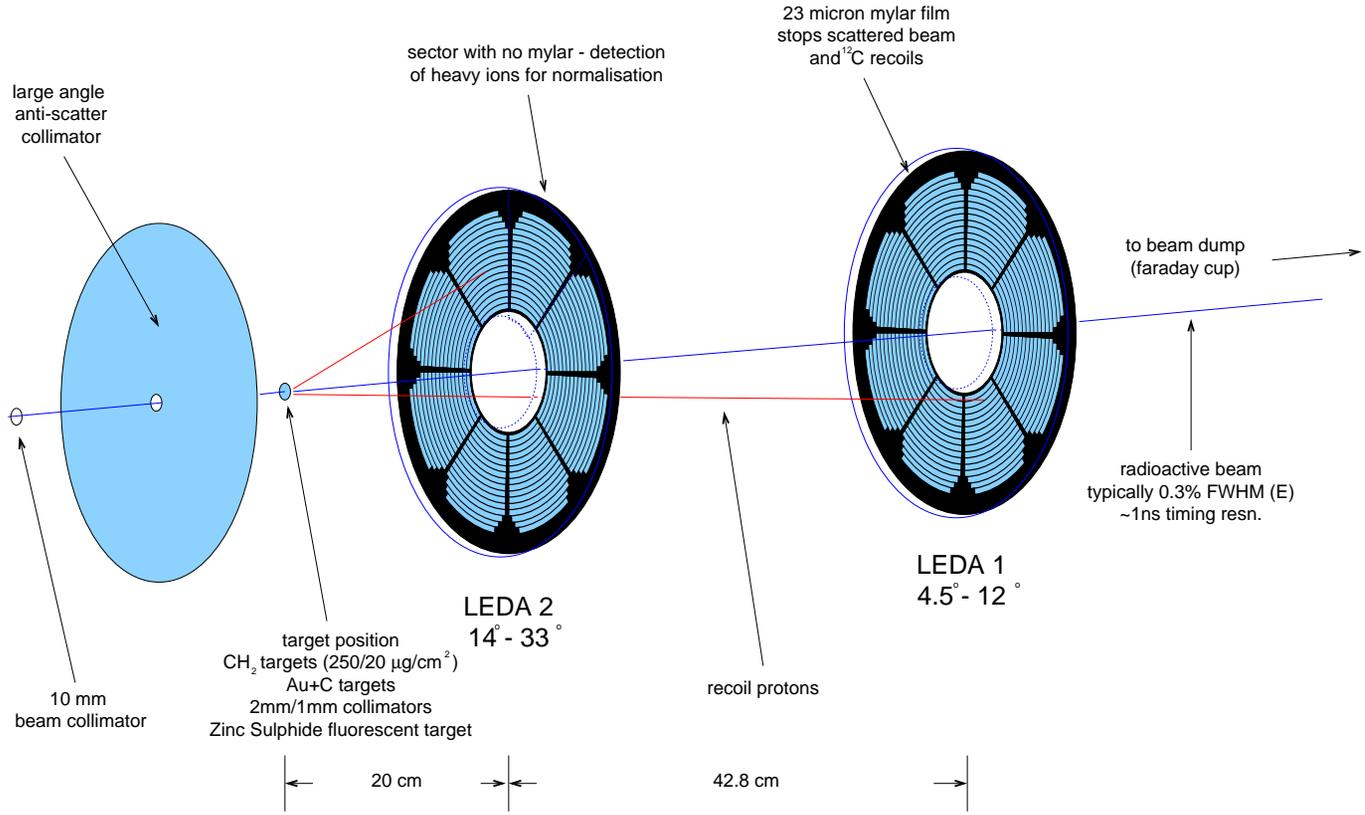
Figure 5.2: Schematic of the experimental setup inside the TUDA chamber.
