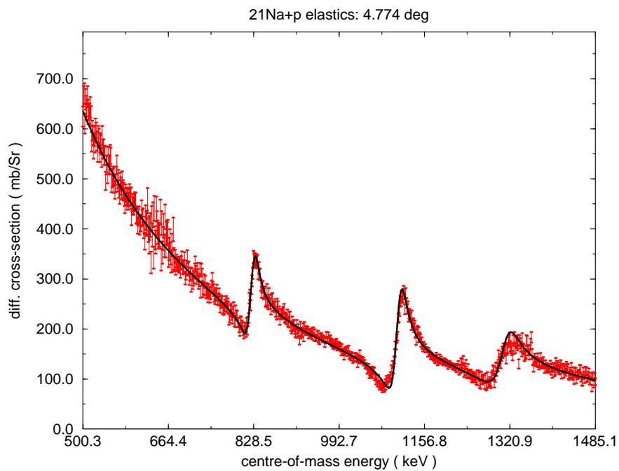
**Figure 7.5:** Single-channel *s*-wave *R*-Matrix fit to  $4.774^\circ$  data using experimental resolution parameters derived from target edges.
